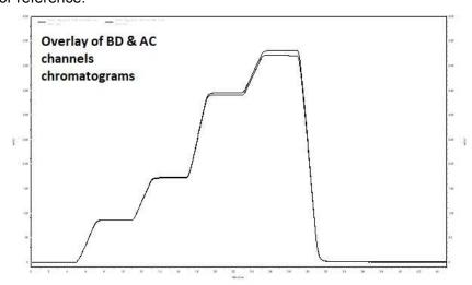
Acceptance Criteria: The gradient profile of A/C and B/D should overlay with each other with difference in absorbance should not more than 0.01 AU and the difference in time should not more than 20 seconds. Chromatogram is attached for reference.
